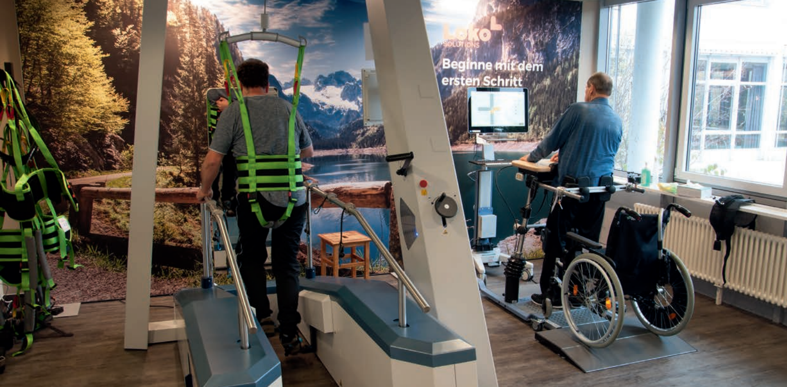
Fig. 1: Picture of a robot-assisted gait trainer, THERA-Trainer lyra. The gait trainer offers a safe, intensive and repetitive locomotion therapy and thus an ideal and cost-efficient training for heavily affected patients post stroke.
